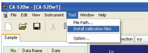
4. When the Insert calibration-DVD message dialog box appears, insert the calibration data DVD in the drive and click the OK button.
